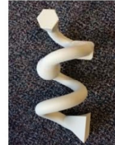
PEKK part produced by OPM T_g + 160\text{ }^\circ\text{C}
